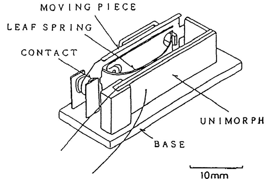
Fig. 9.15 Structure of the latching relay using shape memory ceramic
