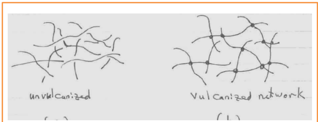
Figure of vulcanized and un-vulcanized rubber molecules
