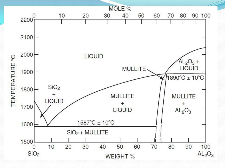
**Superduty** fireclay brick have good strength and volume stability at high temperatures and an alumina content of 40% to 44%. Some superduty brick have superior resistance to cracking or spalling when subjected to rapid changes of temperature.
