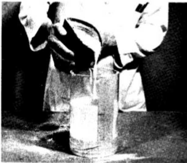
Plaster Node1 Being Poured
