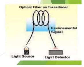
Extrinsic sensors: In contrast to intrinsic sensing, in extrinsic sensing; the fiber may be used as information carriers that lead to a black box and that will generate a light signal depending on the information arrived at black box. This black box may be made of mirrors, gas, liquid cell, or many other mechanisms that will proceed to generate an optical signal.
