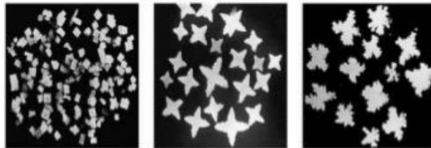
Figure Habit changes in sodium chloride crystals caused by traces of impurity: (a) pure solution, (b) 0.1% \text{Fe}(\text{CN})_6^{4-} , (c) 1% \text{Fe}(\text{CN})_6^{4-} . (Cooke, 1966)
