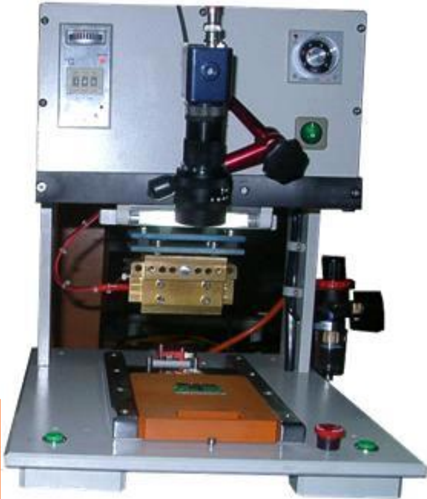
Figure 3. The hot pressing process: schematic of the apparatus.
