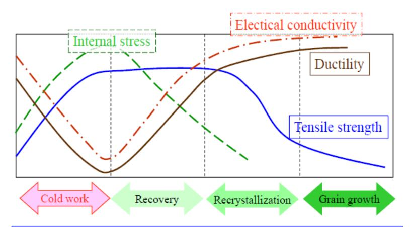
Change of properties with increased annealing temperature of a cold worked sample. Note that there are changes in properties beyond recrystallisation temperatures too due to grain growth.
