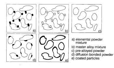
Powder mixtures of elemental or alloy constituents are the easiest way to provide the desired concentration of alloying elements. The advantages of powder mixtures are their versatility and relatively good compactability.
