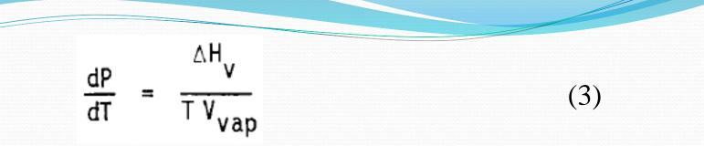
Assuming that the vapour behaves as an ideal gas, the volume  $V_{\text{vap}}$  may be related to
