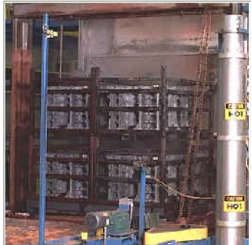
Cylinder Blocks Exiting the Heat Treat Furnace at Alfe Heat Treat, Defiance, OH
