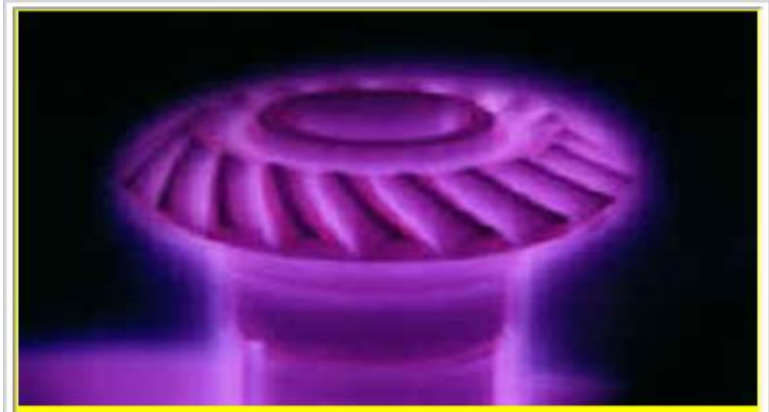
Component in Plasma Nitriding Chamber (from Rubig Plant Technology)
