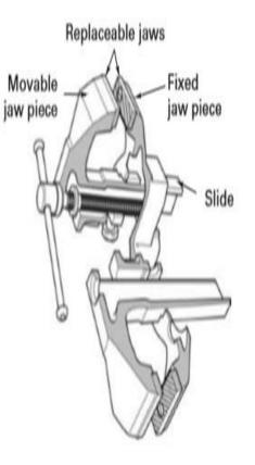
Note: shaded surfaces have been produced by cross-sectional cuts
