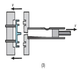
The mold cavity and gating system are machined into the mold and thus become can integral part of it. To produce castings with internal cavities, cores made of metal or sand aggregate are placed in the mold prior to casting.
