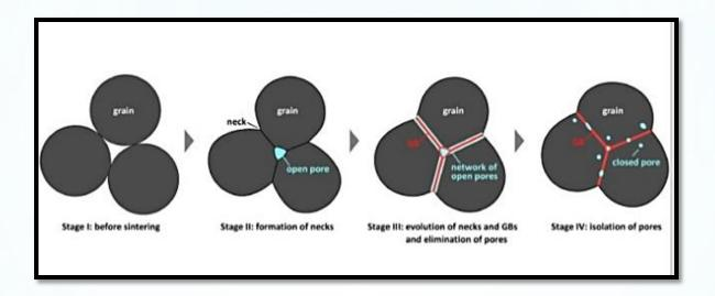
**Fig.(1) Stages of Sintering**
