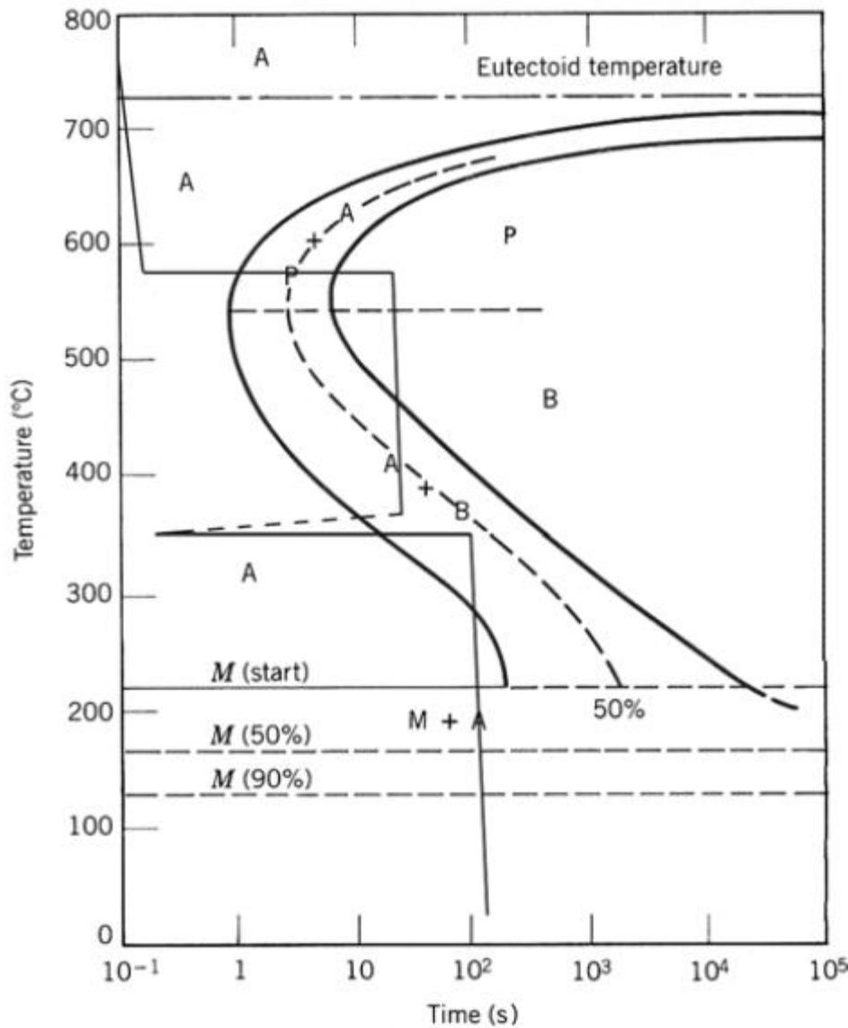
After cooling and holding at  $575^{\circ}\text{C}$  for 20 s, the entire specimen has transformed to fine pearlite. Therefore, during the second heat treatment at  $350^{\circ}\text{C}$  no additional transformations will occur. Hence, the final microstructure consists of 100% fine pearlite.
