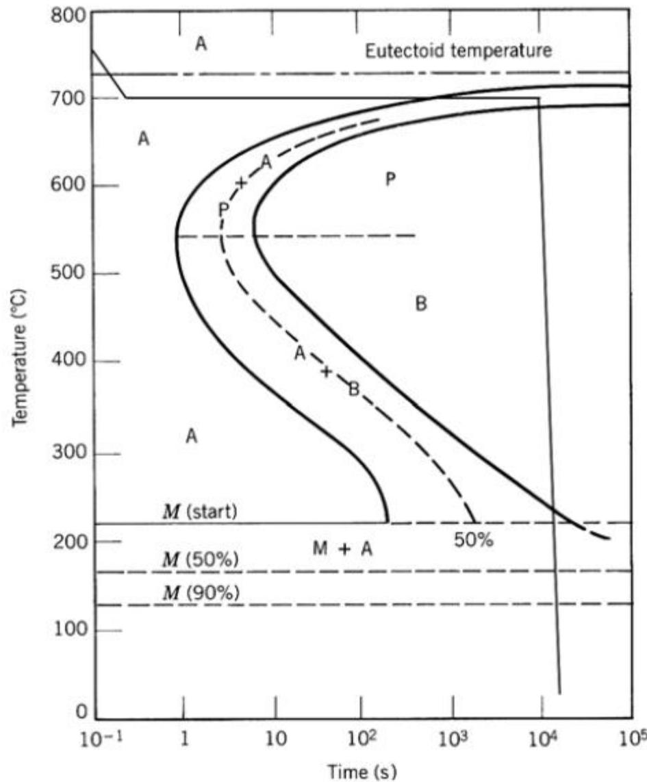
After cooling and holding at  $700^{\circ}\text{C}$  for  $10^4$  s, approximately 50% of the specimen has transformed to coarse pearlite. Upon cooling to room temperature, the remaining 50% transforms to martensite. Hence, the final microstructure consists of about 50% coarse pearlite and 50% martensite.
