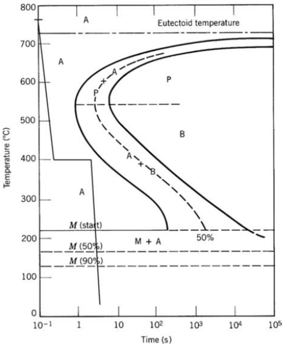
After cooling to and holding at  $400^{\circ}\text{C}$  for 2 s, no of the transformation begin lines have been crossed, and therefore, the specimen is 100% austenite. Upon cooling rapidly to room temperature, all of the specimen transforms to martensite, such that the final microstructure is 100% martensite.
