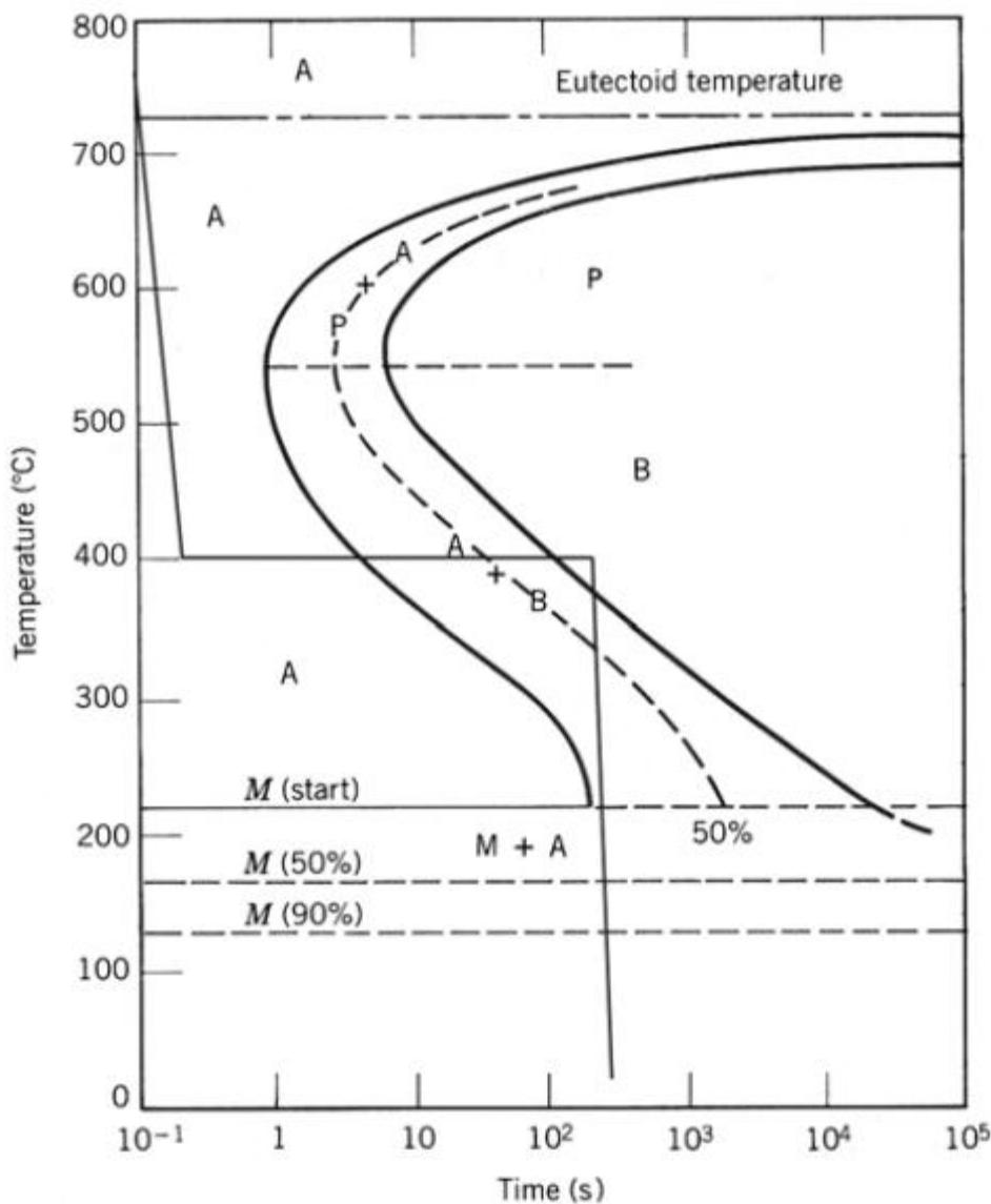
After cooling and holding at  $400^{\circ}\text{C}$  for 200 s, the entire specimen has transformed to bainite. Therefore, during the cooling to room temperature no additional transformations will occur. Hence, the final microstructure consists of 100% bainite.
