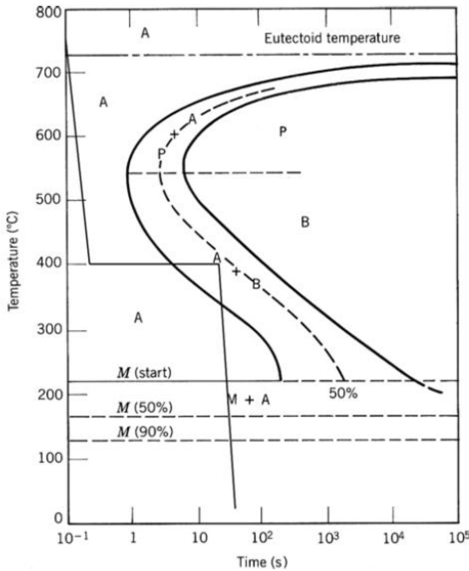
After cooling and holding at  $400^{\circ}\text{C}$  for 20 s, approximately 40% of the specimen has transformed to bainite. Upon cooling to room temperature, the remaining 60% transforms to martensite. Hence, the final microstructure consists of about 40% bainite and 60% martensite.
