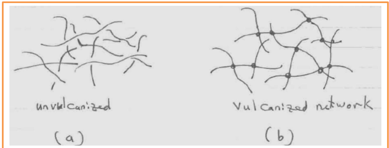
Figure of vulcanized and unvulcanized rubber molecules
