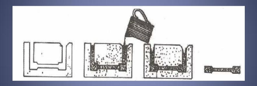
mould Filling mould Absorption of Part removal water from slip
