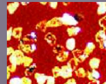
polycrystalline diamonds in a resin matrix.
